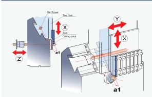
The Y-axis slideway of the tool post incorporates a slanted dovetail structure. The X and Y-axis slideways can be arranged in a pattern close to the cutting point, which improves machine rigidity. In addition, a straight line, passing through the ball screw center which is parallel to the Y-axis slideway and the cutting point are close to each other (a1), reducing the moment load caused by cutting resistance and thereby improving rigidity.
