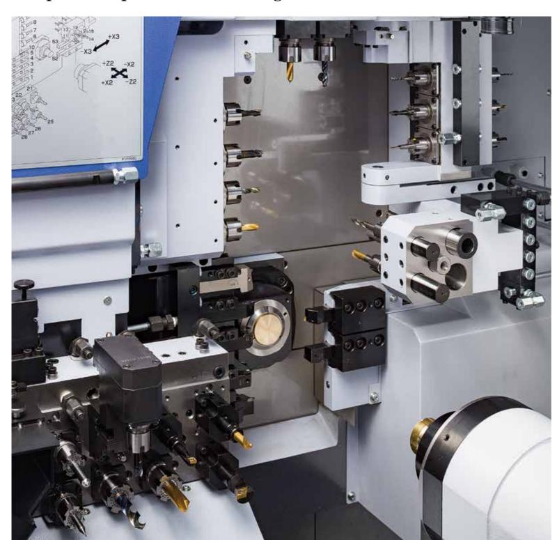
This Quick and versatile multi axis machine offers many functions like balance turning, a fully programmable B axis together with an independent 8-spindle backworking unit for maximum overlapping capability.
