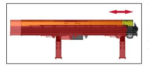
The optional shifting device makes it possible to move the loading magazine up to 400 mm away from the lathe. This practical feature increases accessibility to the lathe for service technicians, e.g. when replacing spindle liners, or, when switching variable lathes from short-turning to longturning mode, ensures the shortest distance between loading magazine and spindle stock at all times.
