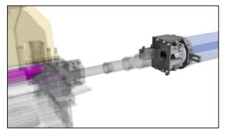
In addition to the use of a telescopic tube, FMB offers a moving steady for lathes with large travel distances along the Z axis and long spindles. This is linked to the spindle stock, thus offering an additional support point for the material bar in order to reduce the free length between the steady and the collet in the lathe. It reduces vibrations in the material bar and has a positive effect on the production quality of the parts.
