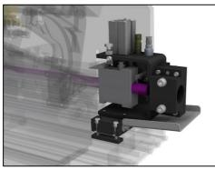
The steady at the end of the guide channel is adjustable and designed with jaws, enabling it to be used for round, square or hexagonal section materials. The steady has easily replaceable (material guides), enabling it to be set to the dimensions of the material bar, thus guaranteeing optimum guidance even of smalldiameter bars in a larger guide channel.
