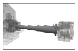
Telescopic tubes are used to bridge the gap when fitting a bar loading magazine to a lathe with a moveable spindle stock. FMB offers an optional package to suit each type of lathe, to ensure secure protection of the rotating bar and the best possible guidance.
