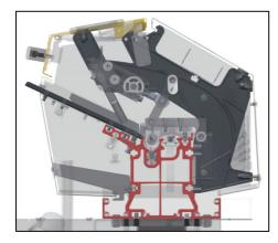
The torsion-resistant machine support of extruded aluminium forms the solid basis for the loading magazine. It also holds the diameter-related inserts for the guide channel.
