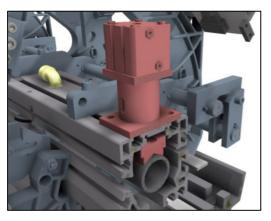
This option is suitable for lathes with a fixed spindle stock. It prevents the pusher from tipping during follow-up and when the collet is open. The pusher is fixed from above in the front area of the channel with 2 pneumatically operated prisms, and prevents the material bar from being clamped off-centre in the chuck. The pusher is also stabilised during the turning process. This method has a positive effect on the quality of the parts produced.
