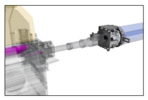
In addition to the use of a telescopic tube, FMB offers a moving steady for lathes with large travel distances along the Z axis and long spindles. This is linked to the spindle stock, thus offering an additional support point for the material bar in order to reduce the free length between the steady and the collet in the lathe. It reduces vibrations in the material bar and has a positive effect on the production quality of the parts.
