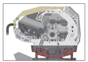
The solid, torsion-resistant machine bed of grey cast iron forms the solid basis for the loading magazine. This guarantees the highest possible guide quality and vibration damping.
