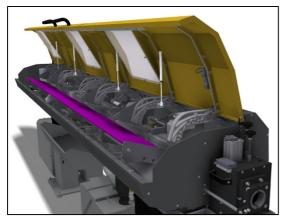
The wide material storage facility offers space for 3 to 48 bars, depending on diameter, in order to allow the lathe to operate for a maximum length of machining time without interruption. The inclination angle of the material storage facility can be infinitely adjusted so that it always guarantees the best possible feed of all kinds of material and profile.
