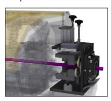
The steady at the end of the guide channel takes the form of a flexible roller steady for the processing of round material bars. When processing round, square and hexagonal section materials the guide rollers can be replaced by appropriate material guides (guide jaws). This enables the steady to be set to the dimensions of the material bar, thus guaranteeing optimum guidance even of small-diameter bars in a larger guide channel.
