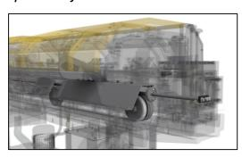
When using a moving spindle stock (e.g. in long-turning mode), the synchronizing device uses a coupling system to couple the bar feed device of the loading magazine mechanically to the spindle stock, thus ensuring synchronisation with the movement of the pusher. As an option, the position during this movement can also be monitored by a sensor to prevent any possible collisions, e.g. when switching from short-turning to long-turning mode.
