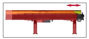
The optional shifting device makes it possible to move the loading magazine up to 400 mm away from the lathe. This practical feature increases accessibility to the lathe for service technicians, e.g. when replacing spindle liners, or, when switching variable lathes from short-turning to long-turning mode, ensures the shortest distance between loading magazine and spindle stock at all times.
