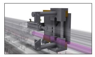
The stable gripper design guarantees secure drawing in of the material bar and removal of the remnant piece.
